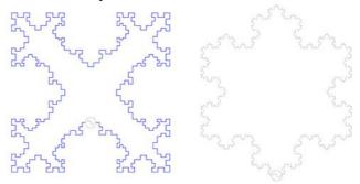
Fig. 3-Two possible fractal loop antennas
