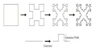
Fig. 6- First three iterations of Minkowski loop
