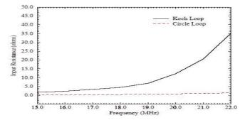
Fig. 5- Input resistances, with regarding to perimeter
