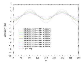
Fig. 7- Far field patterns for resonant fractal loop antennas
