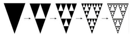
Fig. 8- Generation of Sierpinski sievemethod for computing reflection coefficient
